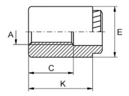
Female thread A = M2 Height K = 12 Hole diameter +0.1 = 3.7 Min distance to edge = 2.2 Min material thickness = 1.5 Outer diameter E = 6 Thread length = 9
